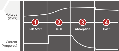
Automatic and High Frequency 4-Stage Charging Curve ■ For all smart charger, apply on Gel and normal battery
